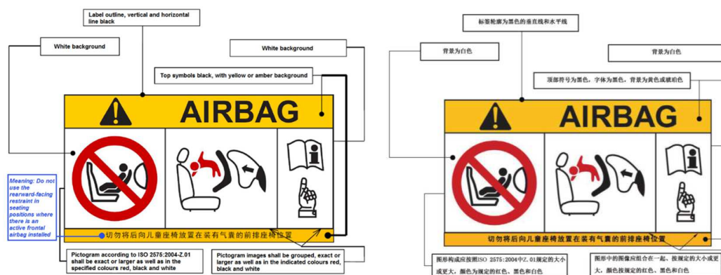
Figure 11 Warning label for rearward-facing restraints 图 11 后向的约束系统的警告标签
