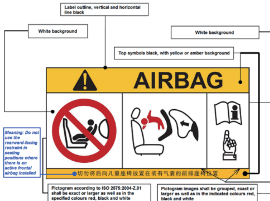
Figure 11 Warning label for rearward-facing restraints后向约束警告标志
